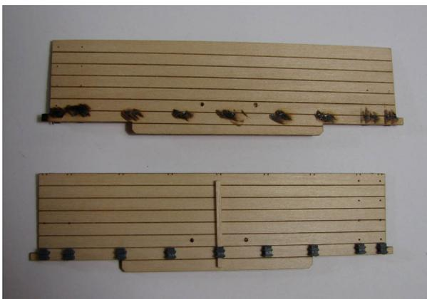
Cut the stakes to length from the bundle of stripwood supplied. Note the two different lengths required, 12 at 1 3/8" and 6 at 1 1/2" and cut the appropriate lengths from their respective package. On the Tweetsie the stakes are 1 1/4" and 1 1/2".
