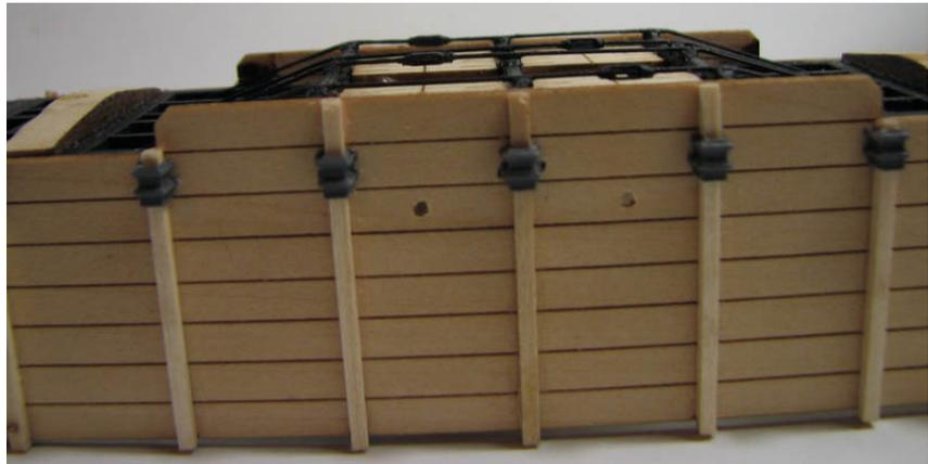
Next, glue the stakes into the pockets and onto the sides. Again, if your boards were cut apart, keep them in the proper order as you reassemble the sides. Keep the stakes perpendicular to the sides as you glue them.
